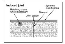
Figure 1: Movement joints
