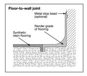
Fig 3: Typical skirting detail
