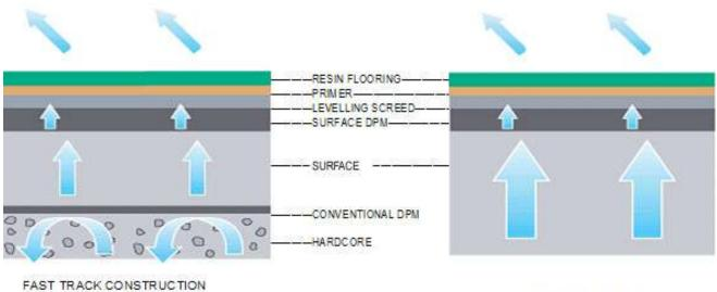
AST TRACK CONSTRUCTION IN THE PRESENCE OF A CONVENTIONAL DPM
